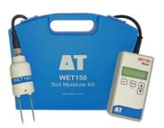
The kit comprises a WET150 Sensor and WET150 Meter. The meter is an easy to use readout-only device (no data recording or other complications) making operation fast and straightforward.
